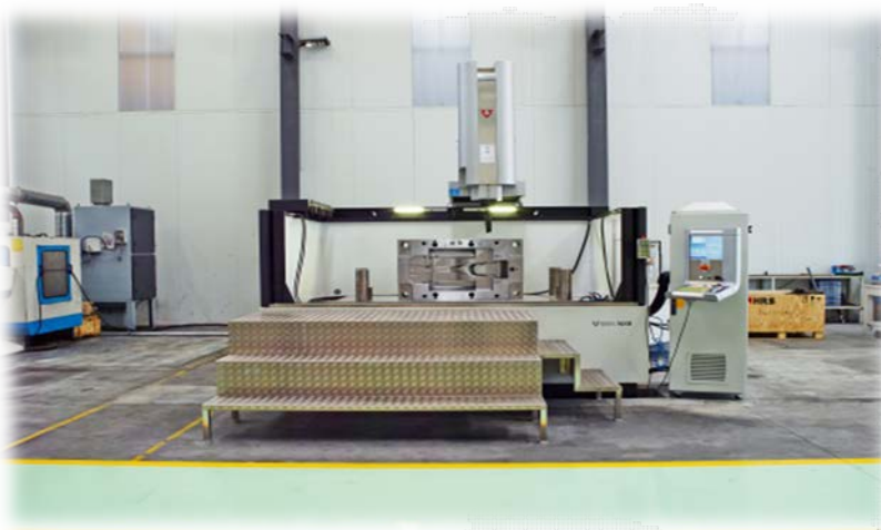
ONA EDM MACHINE Max. Dimensions: X (2000) Y (1000) Z (800)
