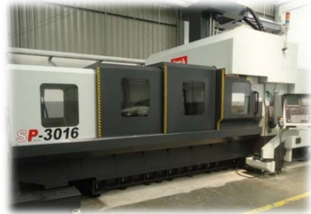
AWEA SP-3016 CNC MILLING MACHINE Max. Dimensions: X (2200) Y (1015) Z (900)
