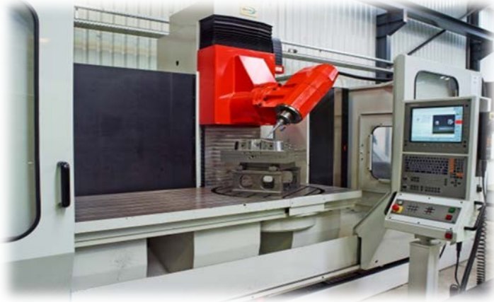
CNC MILLING MACHINE Max. Dimensions: X (2950) Y (1450) Z (1000)
